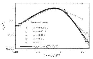
FIG. 5. Nondimensional standard deviation of concentration  $\sigma_c/c_o$  as a function of  $t(\sigma_o^2/\varepsilon)^{1/3}$  for simulated plumes, predicted by the model for five values of  $\sigma_o$ . The solid line represents (32), i.e.,  $\sigma_c/c_o = 1.87\sigma_o^{3/2}\varepsilon^{-3/4}t^{-9/4}$ .
