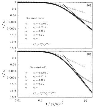
FIG. 4. Nondimensional mean concentration  $\overline{c}/c_o$  as a function of  $t/(\sigma_o^2/\varepsilon)^{1/3}$ , predicted by the model for five values of  $\sigma_o$ : results for (a) simulated plumes and (b) simulated puffs. The solid lines plotted in (a) and (b) represent (28) and (29), i.e.,  $\overline{c}/c_o = C_r^{-1}\sigma_o^2\varepsilon^{-1}t^{-3}$  and  $\overline{c}/c_o = C_r^{-3/2}\sigma_o^2\varepsilon^{-3/2}t^{-9/2}$ , respectively.
