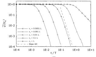
FIG. 1. Mean-square concentration  $\overline{c^2}$  predicted by the model, normalized over the square concentration at the source  $c_o^2$ , plotted as a function of t/T for five values of the source size  $\sigma_o$  ranging from  $10^{-4}$ L to L. The dashed line has a slope equal to -9/2.
