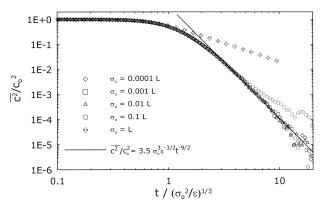
FIG. 2. Nondimensional mean-square concentration  $\overline{c^2/c_o^2}$  as a function of the nondimensional variable  $t/(\sigma_o^2/\varepsilon)^{1/3}$ , predicted by the model for five values of  $\sigma_o$ . The solid line represents (22), i.e.,  $\overline{c^2/c_o^2} = 3.5\sigma_o^3\varepsilon^{-3/2}t^{-9/2}$ .
