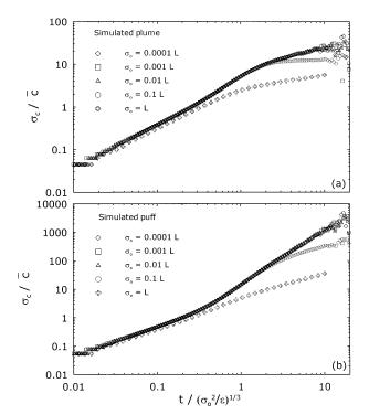
FIG. 6. Intensity of concentration fluctuations  $\sigma_c/\overline{c}$  as a function of  $t/(\sigma_c^2/\varepsilon)^{1/3}$ , predicted by the model for five values of  $\sigma_o$ : results for (a) simulated plumes and (b) simulated puffs.
